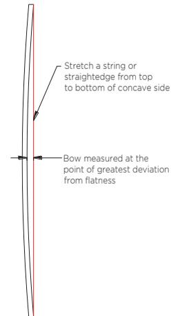
Unusually narrow glass panels, strips, or odd shapes can have an effect that may cause great bow or warp than indicated above. Consult factory for bow and warp tolerance for such items.
